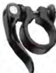
613C672 Material: AL6061. with special bolt & nut to lock. Spec: 31.8 / 34.9. H: 16mm. Color: As order. Standard: Blast anodize
