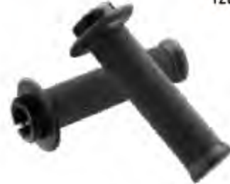
6291376 Material Synthetics Gel. Key Point Double Density. Ø22.4mm W/Flange. Vis G2 One Side Rings. L: 132mm
