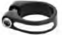
613C681 Diam:28.6,31.8,34.9m/m. Material:AL6061.7005.cold forged
