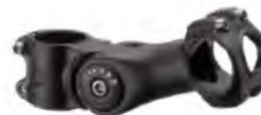
6161157 MATERIAL:FORGED AL6061. ANGLE:40°~140°. EXTENSION:90/110. BAR BORE:MA-595: ø31.8MM. MA-589: ø25.4MM/ ø31.8MM. CLAMP I.D: ø28.6MM/ ø25.4MM. STACK HEIGHT:39MM. ø25.4*128MM. FINISH:BLACK/SILVER/ANODIZED/S.B.COLOR
