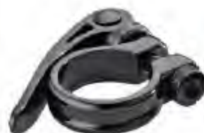
613C653 Diam: 28.6, 31.8, 34.9m / m. Material: AL6061. Cold forged
