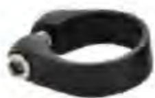
613C684 Diam:28.6,31.8,34.9m/m. Material:AL6061.7005.cold forged
