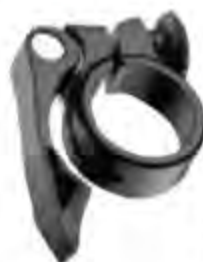
613C672 Material: AL6061. with special bolt & nut to lock. Spec: 31.8 / 34.9. H: 16mm. Color: As order. Standard: Blast anodize
