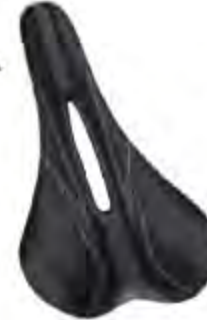
6281209 Size: 274 x 134mm Base: Carbon Fiber injection, Nylon Fiber injection. Fill: Light foam High Density. Rail: Crn-Ti Alloy, Chromoly Steel.
