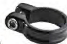
613C668 Diam: 28.6, 31.8, 34.9m / m. Material: AL6061. cold forged
