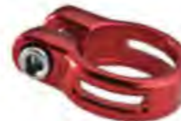
613C655 Diam: 28.6, 31.8, 34.9 m / m. Material: AL6061. cold forged
