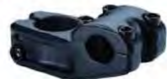
616121 Malt-forged/ Forged Cap. 28.6*50mm. Bar Bore: 22.2mm. Angle: 0°. Stack Height: 30mm
