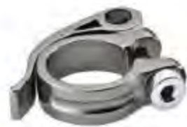
613C652 Diam: 28.6, 31.8, 34.9 m / m. Material: AL6061. cold forged
