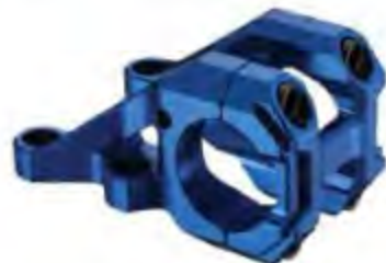
616118 Material: fully Cnc-machined 6061 T6 Alloy. Bar bore: 31.8/34.9mm. Extension: 50mm. Angle: 0°
