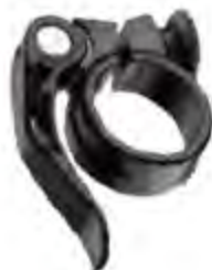
613C671 Material: AL6061. with special bolt & nut to lock. Spec: 31.8 / 34.9. H: 16mm. Color: As order. Standard: Blast anodize
