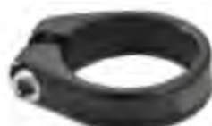
613C685 Material: AL6061 cold forged Size: 28.6,31.8,34.9mm
