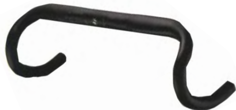
615795 Material: AL6061/ AL7075 butted. Center Dia: 31.8. W: 400/420/440 mm, Drop: 155, Reach: 98.5, Finish: Mat Bk.
