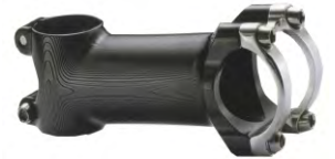
6161023 Full set 3D CNC machined body & front cover. 7050 w/ stainless bolts . Ext: 80~130. Angle : ±5°. Bar bore: 31.80 Dia: 28.6. H: 39mm. Finish: anodized. EXT: 100mm
