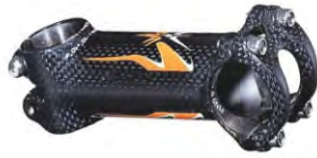
6161021 Bar bore: 31.8. AL2014+ Carbon skin. Angle: -6° / +6°. Ext: 90,100,110,120 mm. L: 38 mm. Dia: 28.6mm
