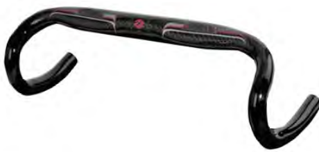
615790 Material: Alloy + carbon. Diameter: \phi 31.8. Width: 400 420 440. Reach: 80. Drop: 125. Finish: MCF GCF. Weight: 360g (W:420)
