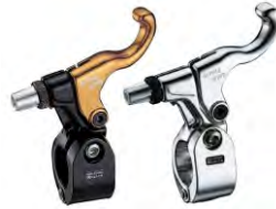
617L848 Forged alum bracket (Anodized powder white or pink). Forged alum lever handle (Anodized)Double bent lever handle for Dirt jump. Hinged clamp. Clamp 25.4mm standard or w/sleeve for 22.2mm handle bar. Usable on curve position (Short handle bar).
