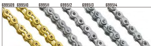
699509 / 699510 / 699511 / 699512 / 699513 / 699514 Size: 1/2" x 3/32". 1/2" x 1/8". 1/2" x 3/16". Color: Gold, silver, silver/black, gray/gray Compatible bikes: BMX, Freestyle, Beach cruiser. Special dynamic configuration plates. Light weight & stretch proof hollow pin. Stretch proof mushroomed pin, enhanced durability. Anti-drop design
