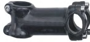
6161022 EN-M/EN-R approved. 3D forged stem. L: 70/80/90/100/110/120mm. Angle: 7 degree. Dia: 25.4/26.0mm Steerer : 25.4/28.6mm. H: 41mm. Finish: anodized
