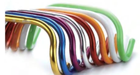
615799 Material: AL6061. Center dia: \phi 25.4, \phi 26.0, \phi 31.8 Width: 370/380/400/420/440. Drop (D): 169mm. Reach (R): 101mm. Weight: 299g. ( \phi 31.8 W:400 AL6061) Finish: SHINY BK, SHINY SV, MAT SV, P.WH, CP, MAS, MSBK
