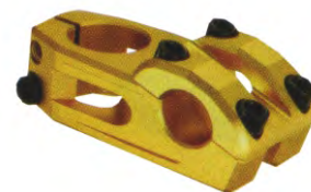
6161039 Extrusion with full CNC. 28.6 X 53mm. Bar bore: 22.2mm. Angle: 0°. H: 30mm
