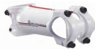
6161029 3D forged / 7075-T6 alum 2014 alloy faceplate. Stainless steel hardware. L: 60~130mm. Angle: +/- 7 degree. Dia: 31.8mm. Steerer : 28.6mm
