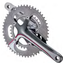
610812 Integrated outside bearing B.B. Chainring: 53T/39T teeth (7075/T6) CNC. Crank: Forged 6061/T6 alloy. L: 165, 170, 172.5, 175mm. BCD: 130mm
