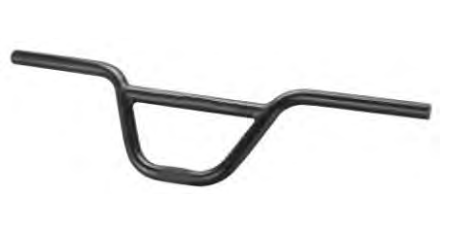
615800 Material: Alloy. Bar bore: \phi 22.2mm. Up sweep: 2° Back sweep: 8° Width: 625 mm. Weight: 413g. Finish: Black/silver/anodized/S.B color
