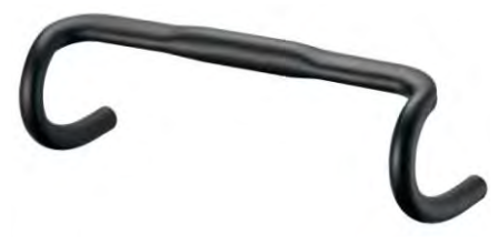
615797 Material: Alloy. Bar bore: \phi 31.8mm. Reach: 80mm. Drop: 120mm. Width: 380/400/420/440mm. Weight: 375g. 440mm. Finish: Black/silver/anodized/ S.B color
