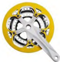
610822 Crank: Forged Alloy 6061 Crank Finish: Hi-polish Black/Silver Chain Ring: 52T/42T/30T BCD: 130/74. Crank L: 175/170 mm. Chain Guard: Alloy
