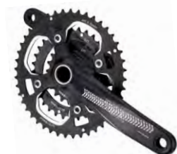
610811 Chainring: 22/32/42T, 22/32/44T, 28/38/48T. Crank: Forged 6061/T6 alloy. L: 170, 175mm. BCD: 104/64mm
