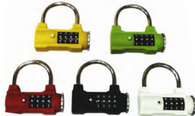
641841 4 digit resettable combination padlock. Elastomeric paint lock body cover. Lock body cover covers the dials wheel. Shackle dia 8mm, hardened
