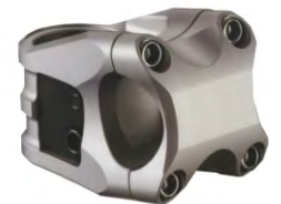
6161035 Fully CNC-machined 6061 T6 alloy. Bar/ Dia: 25.4 / 31.8mm. Extension: 45mm. Steerer: 28.6mm. Angle : 0°. H: 41 mm
