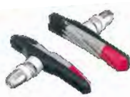
618921 Anodized black pad holder. Triple color compound. L: 72mm
