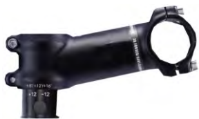
6161032 3D Forged / 6061-T6 aluminum. Alloy Faceplate. L70/80/100/110/120mm. 31.8mm diameter. 28.6mm steerer clamp. Finished: S.B Black.
