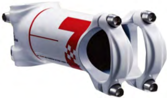
6161024 The new UL stem with 7050 aluminum Weight : 87g (L:90mm (Ti-bolts) Length : 80/90/100/110/120/130mm Angle : +/- 7 degree Diameter : 31.8mm Finished : Carbon/matt black/porcelain/ebony
