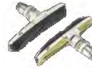
618928 CNC Machined. Threaded Type for V-brake. Alum Pad holder Black Color & Anodized White/Gold. Length: 72mm
