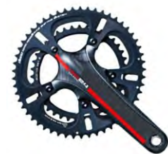
610821 L: 165, 170, 172.5, 175mm. BCD: 110mm. Chainring: 50/34T. Chain line: 43.5mm. Crank W: 615 grams. BB Cups: BC-1.37x24/68 mm. Weight: 95grams
