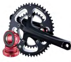
610808 Material: AL-7075/ 7050. BCD: 110mm. Chainring: 50T X 34T. Finish-beadblast / matte black
