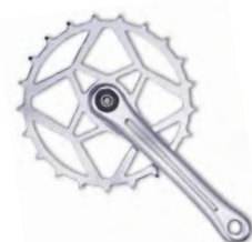
610823 44T, 42T. Skip teeth design. 6061 forged AL crank. 175,170,165mm / riveted
