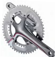
610813 Integrated outside bearing B.B. Chainring: 50/34T teeth (7075/T6) CNC. Crank: Forged 6061/T6 alloy. L: 165, 170, 172.5, 175mm. BCD: 110mm
