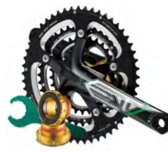
610809 Material: AL-7075 / 7050. BCD : 130 mm. Chainring: 52T X 39T X 30T ; 50T X 39T X 30T. Finish-high polished, silver / black / grey
