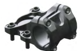
6161040 Alloy 6061 fully CNC machined. Ext: 45/50mm. Bar bore: 31.8mm. Angle: 0°
