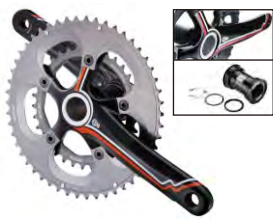
610807 Integrated outside bearing B.B.3D Chainring: 50/34T teeth (7075/T6) CNC Crank: Forged 6061/T6 alloy. Length: 170, 172.5, 175mm. BCD: 110mm
