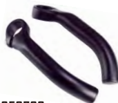
658730 3-D forged one-piece 6061 T6 alloy. L: 105/120mm. Dia: 22.2mm.
