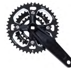
610819 Chainring: 22/32/42T, 22/32/44T, 28/38/48T. Crank: Forged 6061/T6 alloy. Length: 170, 175mm. BCD: 104/64mm
