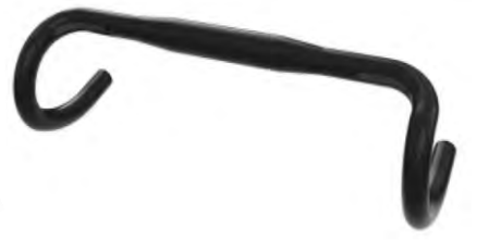
615796 Material: Alloy. Bar bore: \phi 31.8mm. Reach: 80mm. Drop: 120mm. Width: 380/400/420/440mm. Weight: 375g. 440mm. Finish: Black/silver/anodized/ S.B color
