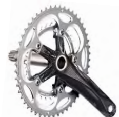
610816 L: 165, 170, 172.5, 175mm. BCD: 110mm Chainring: 50/34T. Chainline: 43.5mm Crank W: 730grams. BB Cups: BC-1.37 x 24/68mm. BB Axle: Cromoly SCM435 Weight: 120grams
