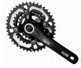
610820 BCD: 104/64mm 4Arm alloy forged crank Crank L: 170, 175mm. Chainring/speed: 306: 42/32/24T(10S), 304: 44/32/22(9S) Material: Outer/CNC, middle: CNC, Inner: CNC/alloy option. Chainline: 50mm BB-B83002 / BB-PF-3002
