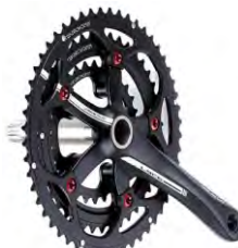
610817 L: 165, 170, 172.5, 175mm. BCD:130/74 mm. Chainring: 52/42/30T. Chainline: 45mm. Crank W: 85grams. BB Cups: BC-1.37 x 24/68mm. BB Axle: Cromoly SCM435. W: 98grams
