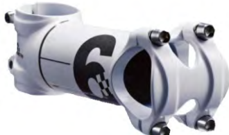
6161025 The new UL stem with 6061 aluminum Weight : 105g/ext. 90mm Ext.60-130mm Angle : +/- 7 degree Diameter : 31.8mm Finished : Matt black/porcelain/ebony
