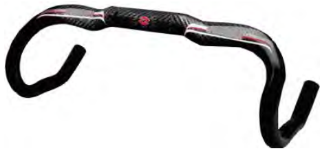
615789 Material: Alloy butted. Diameter: \phi 31.8 Width: 400 420 440. Reach: 103. Drop: 152 Finish: Anodized colors. Weight: 334g (W:420)
