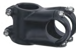
6161034 EN-M/EN-R approved 3D forged stem. L: 70/80/90/100/110/120mm. Angle: 7 degree . Dia: 25.4/ 26.0mm. H: 41mm. Finished: anodized
