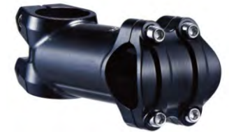
6161027 EN-M/EN-R approved. Die Cast Stem. Angle: 7 degree. Diameter: 31.8mm. Steerer: 28.6mm, Height:42mm. Length: 300/350/400mm. Weight:180g Finished: Barrel Silver, Ed Black.
