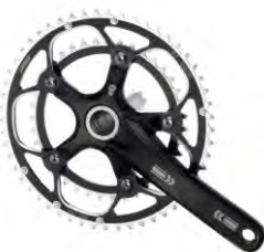
610818 BCD: 130mm 5Arm Alloy forged crank Crank L: 170, 172.5, 175mm. Chainring/speed: 208: 53/39T(9/10S) 209: 52/39T (9/10S) 225: 50/39T(10S) Material: Outer: CNC, Inner: CNC/alloy option. Chainline: 43.5mm. BB-B83001/BB-PF3001
