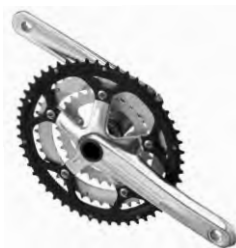
610814 BCD: 130/74mm 5Arm alloy forged crank. Crank L: 170, 172.5, 175 mm. Chainring/speed: 302: 52/42/30T (8/9S) Material: Outer/Middle/Inner: Alloy/Steel Option. Chainline: 45.5mm. BB-EB2401/ BB-B88601
