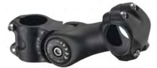
6161031 Material: 6061 forged alloy. Angle 40 - 140. Extension 108/128mm. Bar bore 25.4/31.8mm. Clamp L.D: 25.4/28.6mm Weight: 128mm Finish : Black/Silver/Anodized/S.B color.
