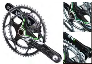
610806 Integrated outside bearing B.B. Chainring: 53/39T teeth (7075/T6) CNC. Crank: Hollow carbon. Length: 170, 172.5, 175mm. BCD:130mm
