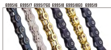
699516 Heavy-duty 1/2" x 1/8" Pin L: 9.20mm. Tensile strength (Min): 1,100 kgf. Color or plates (outer/inner): Dark blue / dark blue. Compatible: Single speed bikes, track bikes. BMX, Freestyle, ATB, Fixed gear 699517 Hollow plate. Pin L: 9.20mm. Tensile strength (Min): 1,100kgf. Color of plates (outer/inner): silver / silver Compatible: Single speed bikes, track bikes, BMX, Freestyle, ATB, Racing, Fixed gear 699518 / 699519 Half-link chain. Pin L: 10.50mm. Tensile strength (Min): 1200 kgf. Color of plates (outer/inner): Dark blue/Dark blue. Compatible: Single speed bikes, track bikes, BMX, Freestyle, ATB, Fixed gear
